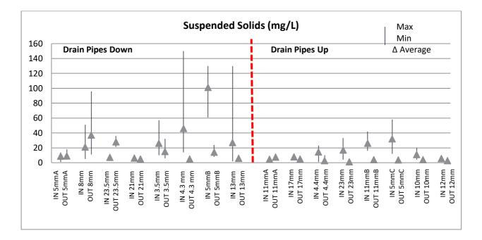
The box plot shows paired values for suspended solids at the inflow and outflow of the biofilter.
