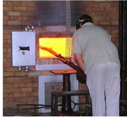
Liquid gold that has been smelted in an arc furnace is removed to pour (demonstration in South Africa) (D Brown 2006, Wikimedia Creative Commons)
