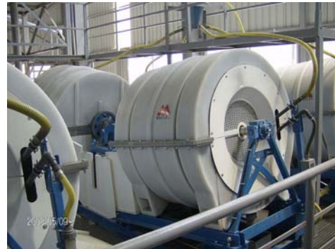
Multi Gravity Separator manufactured by Gravity Mining Ltd, England (2008, Wikimedia Creative Commons)
