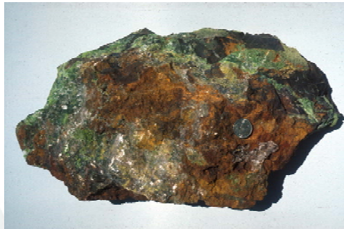
Gossan of nickel-sulphide ore Otter Shoot, Kambalda, WA by R Hill. CSIRO Science Image
