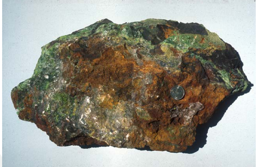
Gossan of nickel-sulphide ore Otter Shoot, Kambalda, WA by R Hill. CSIRO Science Image
