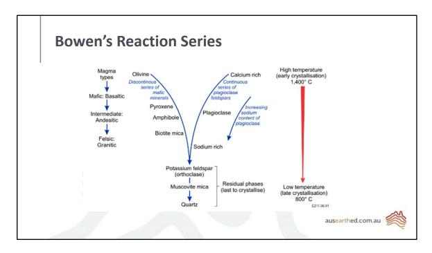
Bowen's Reaction Series, outlined in the early 1900's, assists us to understand the order of crystallisation of the common silicate minerals from a magma.
