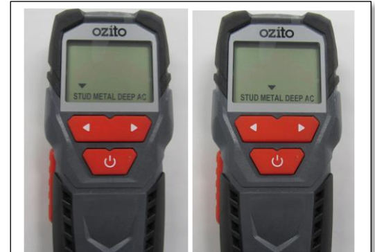
Figure 4: Stud finder needs to have both stud (left) and metal (right) settings.
