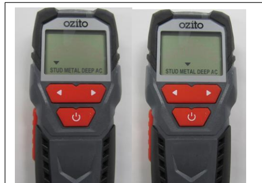
Figure 1: Stud finder needs to have both stud (left) and metal (right) settings.
