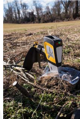
XRF used to measure metal contaminants in soil (L Cheung/ USDA 2018, public domain)
