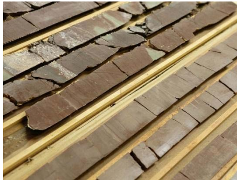
Figure 3: Reservoir core sample, sandstone. (from dea-group.cpm)
