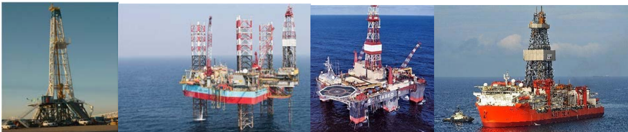
Figure 1: From left to right; Onshore rig ( foxoildrilling.com ), jack-up ( offshore.fleet.com ), semi-submersible ( km.konsberg.com ) and drill ship ( ships.lv )
