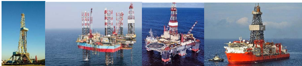
Figure 1: From left to right; Onshore rig, jack-up, semi-submersible and drill ship.
