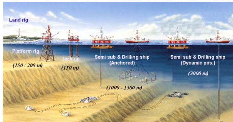
Figure 2: Water depth drilling rigs and ships can operate in.
