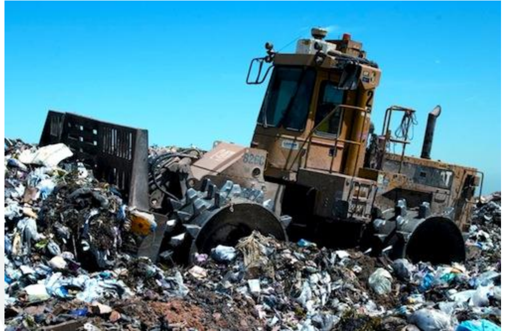
Landfill compactor (2013, public domain)
