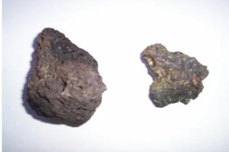
The rock on the left is sinter (siliceous slag) from a recent blast furnace in NSW. The rock on the right was spewed out in 1984 from a volcano in Iceland named Krafla. Both are silica rich, were full of gas when molten and were rapidly cooled at the Earth's surface. Large scale bedding seen in coastal dunes is similar to that demonstrated in the red Bassendean sands which are used by the construction industry in Perth. The Bassendean sands are about 240,000 years old.
