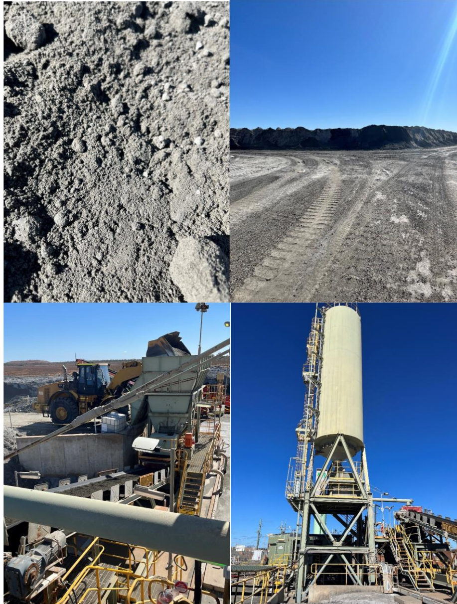
From top left to bottom right: close view of dried tailings; dried tailings stockpile; dry tailings are loaded into a hopper; cement from the large cylinder is mixed with tailings in a 1:21, cement : tailings ratio (photos courtesy of Evolution Mining)
