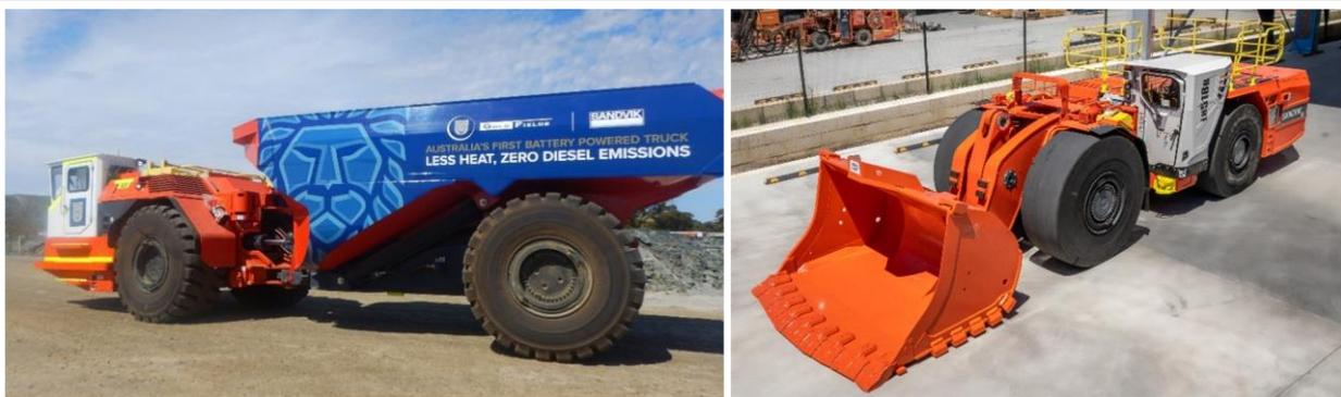
Battery electric underground haul truck (L) and loader (R) being trialed at St Ives Gold Mine. (photos courtesy of Gold Fields)
