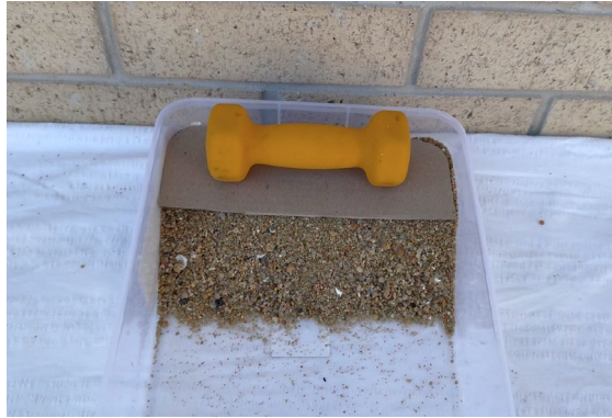
Figure 9: cap applied to piles and load applied. Slope has not collapsed
