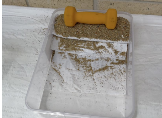
Figure 6: Fabric strips layered in the sand with load applied. Slope has not collapsed
