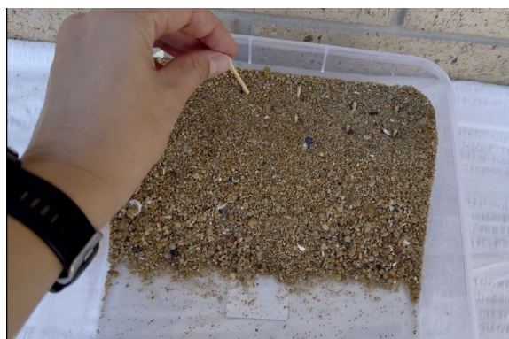
Figure 8: Inserting 'piles' vertically
