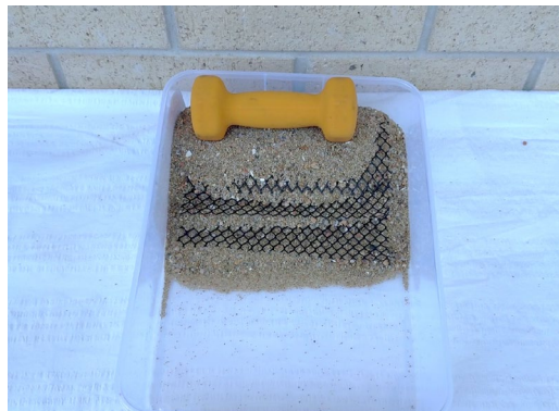
Figure 7: mesh placed in sand with load applied. Slope has not collapsed
