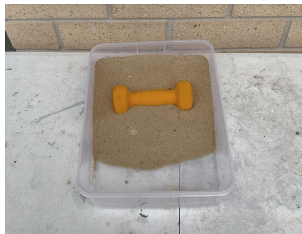
Figure 5: load applied to the slope. Slope has collapsed
