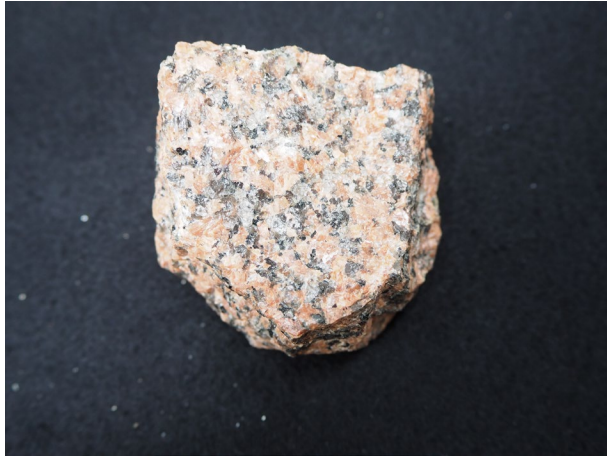
Figure 2: Granite (light in colour, coarse-grained, interlocking crystals)
