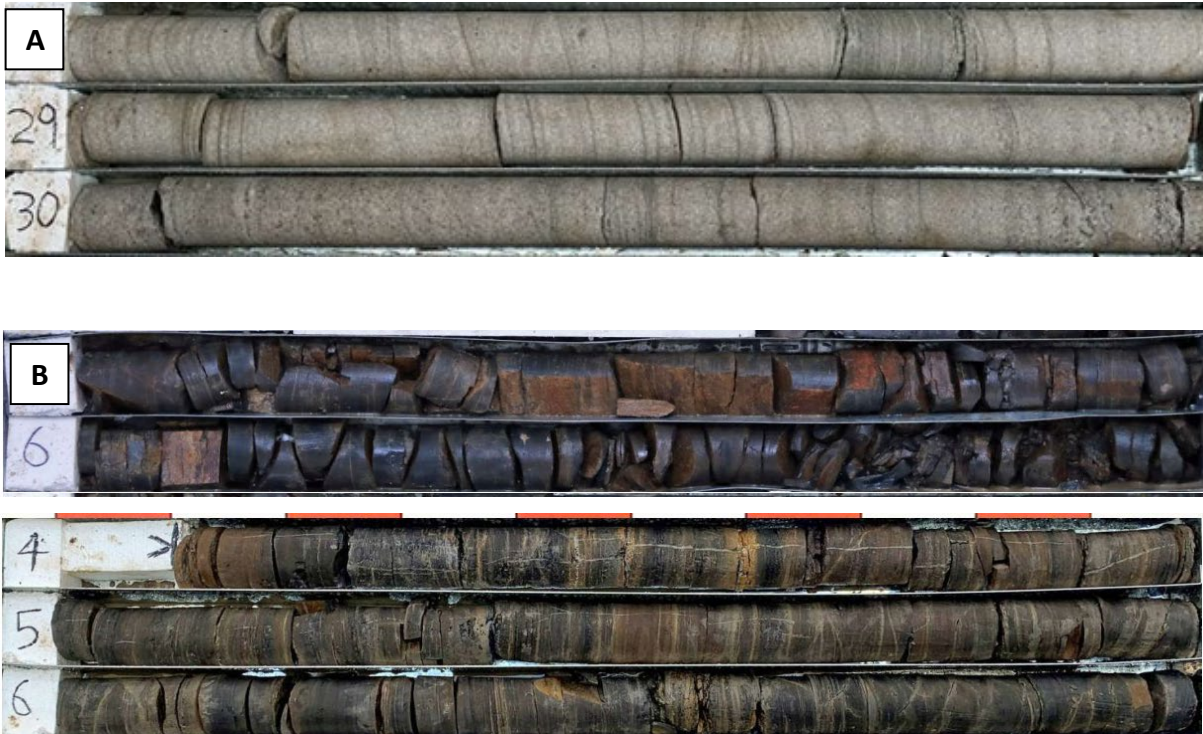
Figure 11: Drill core samples from a geotechnical investigation showing the effect of weathering on rock strength: (A) fresh sandstone core (high strength, intact) and (B) highly weathered siltstone core (very low strength, fragmented). Image: Ali Parsa, JK Geotechnics.
