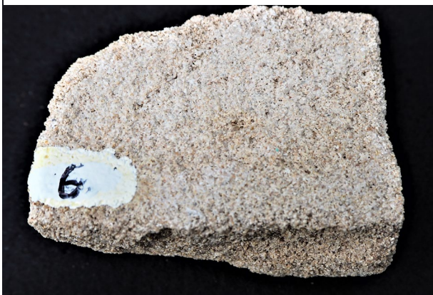
Figure 4: Limestone (range of appearances but usually beige to grey in colour, contains calcium carbonate – use acid test to confirm)
