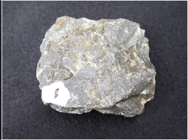
Figure 3: Basalt (dark in colour, fine-grained, interlocking crystals)
