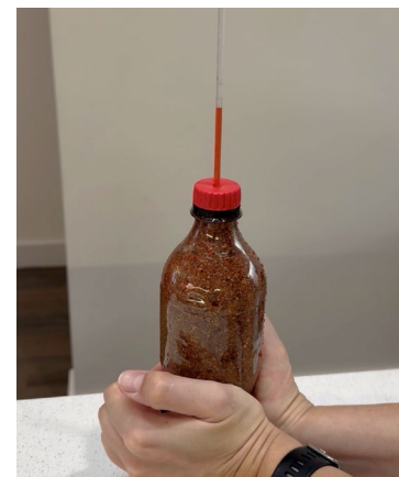
Figure 4: squeezing a bottle containing water-saturated coarse sand
